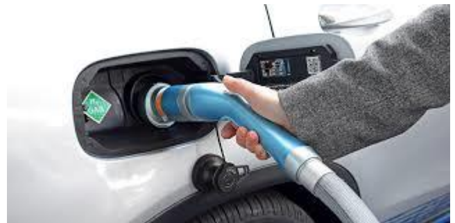
Hydrogen Refuelling Process
