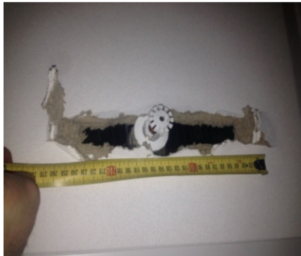
Figure 10: Relative movement of sprinkler and ceiling
