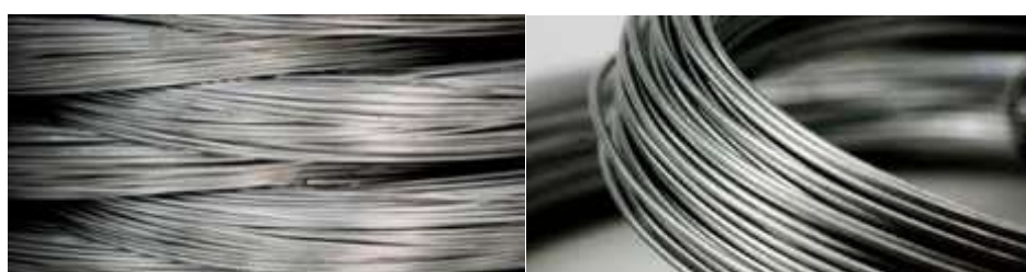
Figure 2.1: Galvanised wire Left: Fencing wire; Right: Manufacturing wire 2
