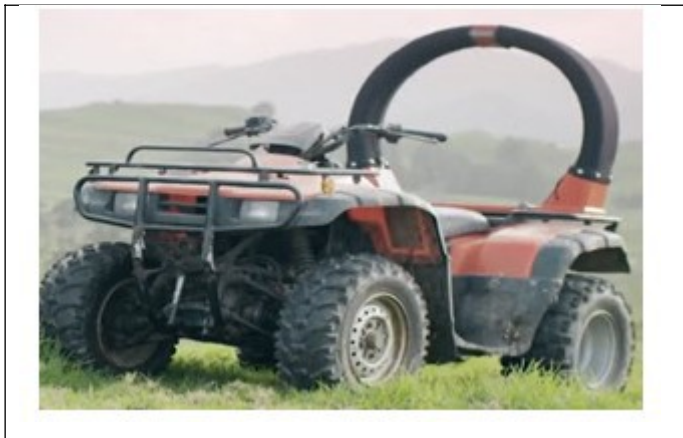
Figure 4: Illustration of roll-over/crush protection device on a quad bike
