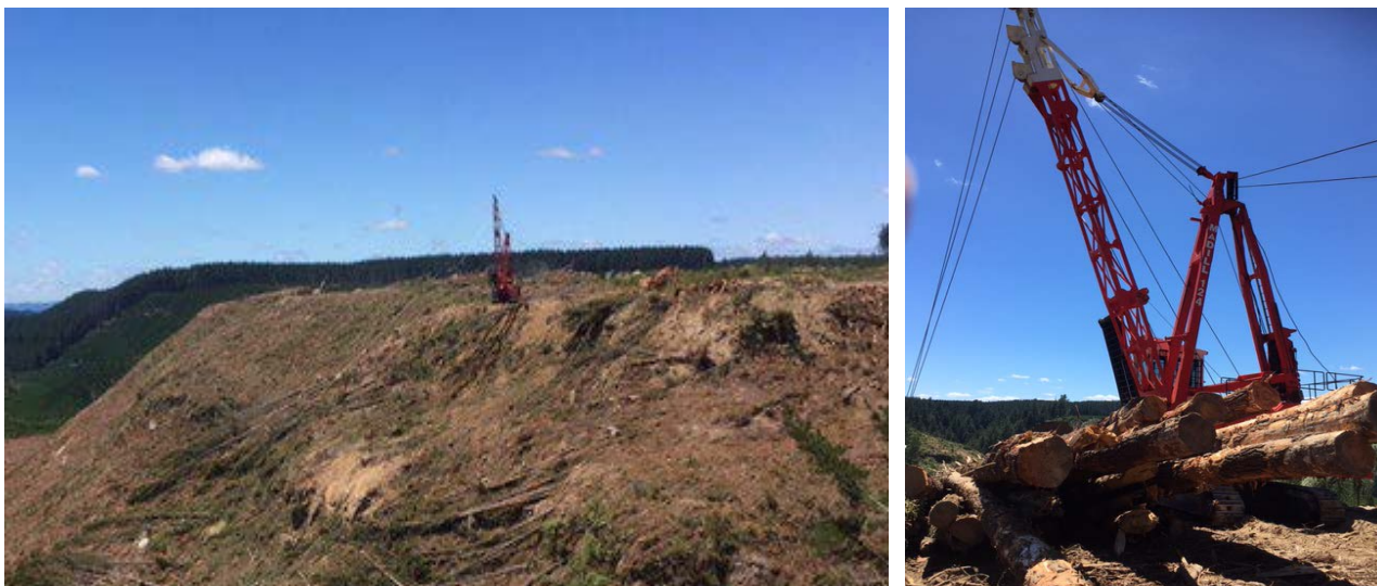
Figure 2 – Illustrations of a cable logging yarder/hauler
