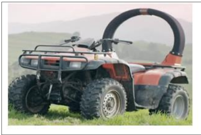
Figure 4: Illustration of roll-over/crush protection device on a quad bike
