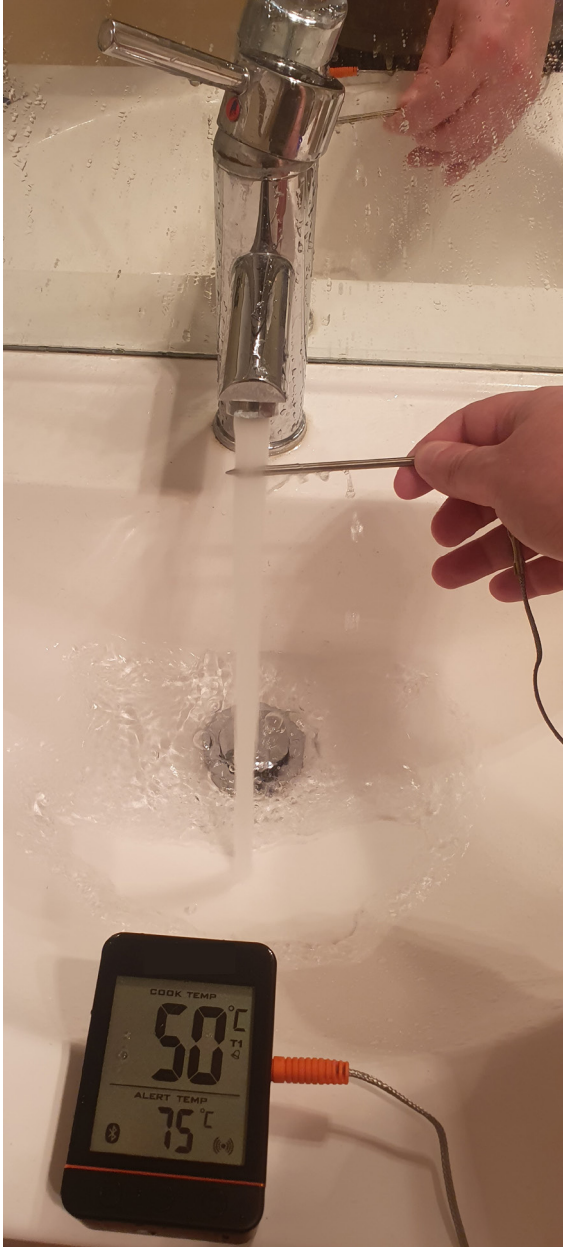
FIGURE 2.1: 50°C – Proposed max temperature of hot water delivered to new bathroom fixtures in homes.
