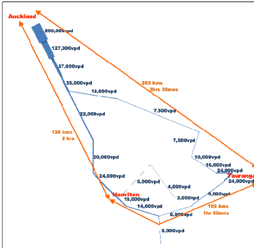
Map A3.1 Traffic volumes (vehicles per day) on key road links within the AHT region.
