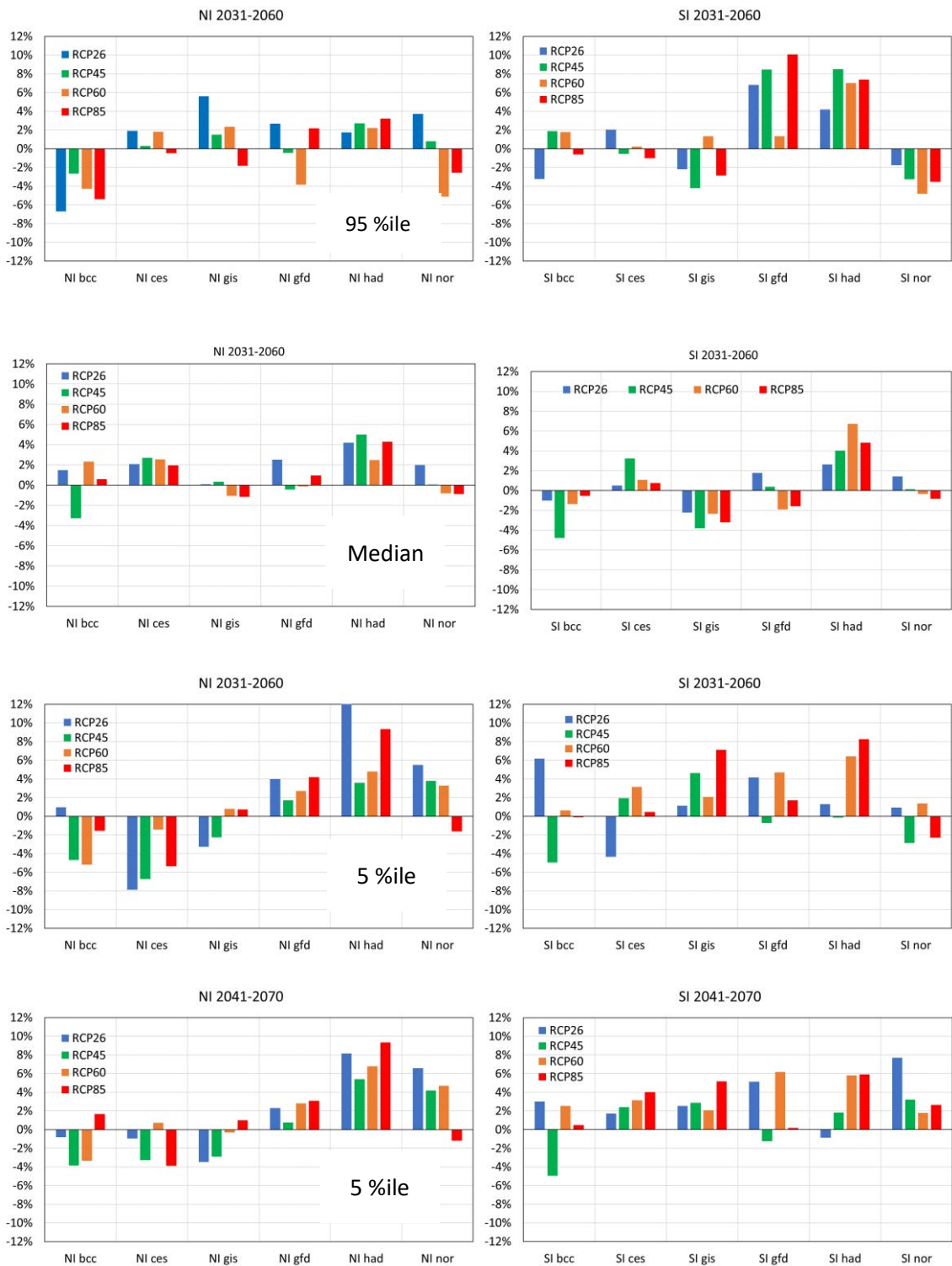
Figure 5-8: Per cent changes (2031 to 2060 vs 1981–2005) in wind generation for each RCP scenario grouped by the six CMIP5 models. The left-hand column is for the North Island and the right-hand side the South Island. The upper panel is for the 95 th percentile (i.e., high generation months exceeded 5% of the time), the second row is for median generation (exceeded 50% of the time), the bottom two rows are for the 5 th percentile (i.e., low production months) for 2031–2060 and 2041–2070 respectively.
