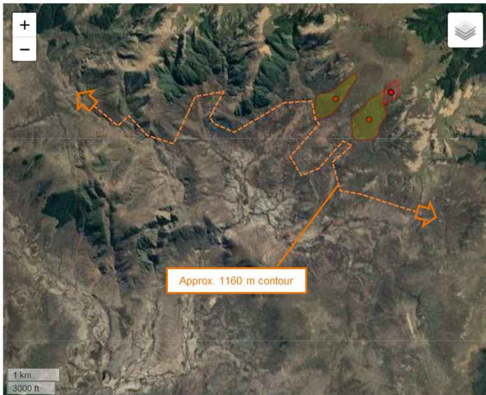
Figure 14 - Mapped area of landsliding on the shoreline of proposed reservoir (from GNS)
