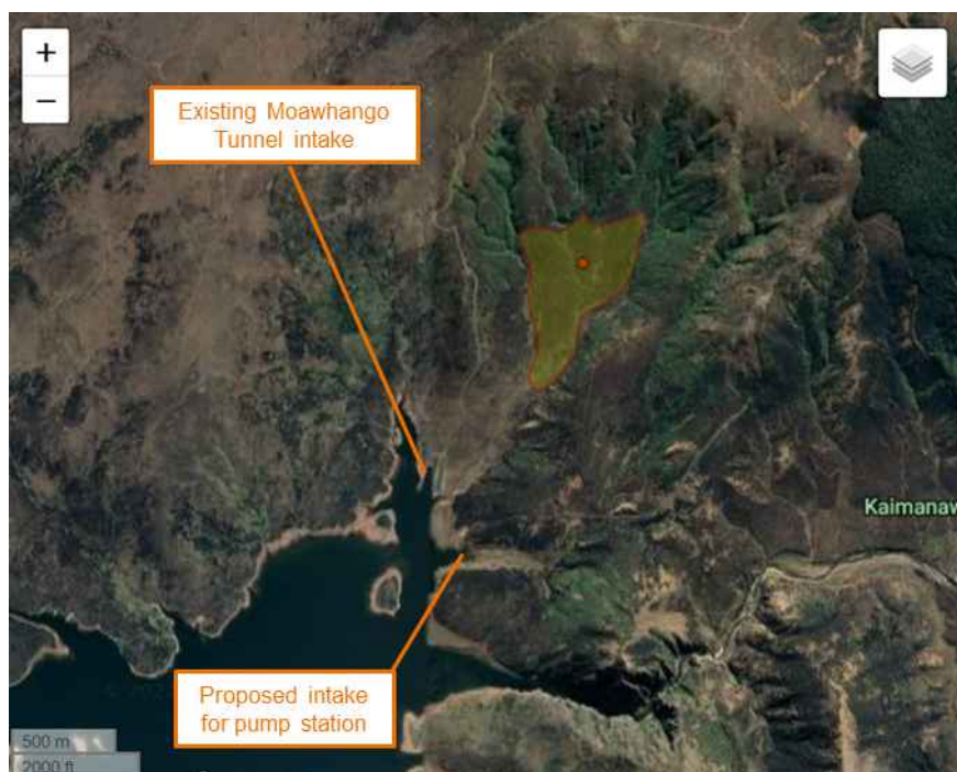
Figure 13 - Mapped area of landsliding on the northern side of Lake Moawhango (from GNS)
