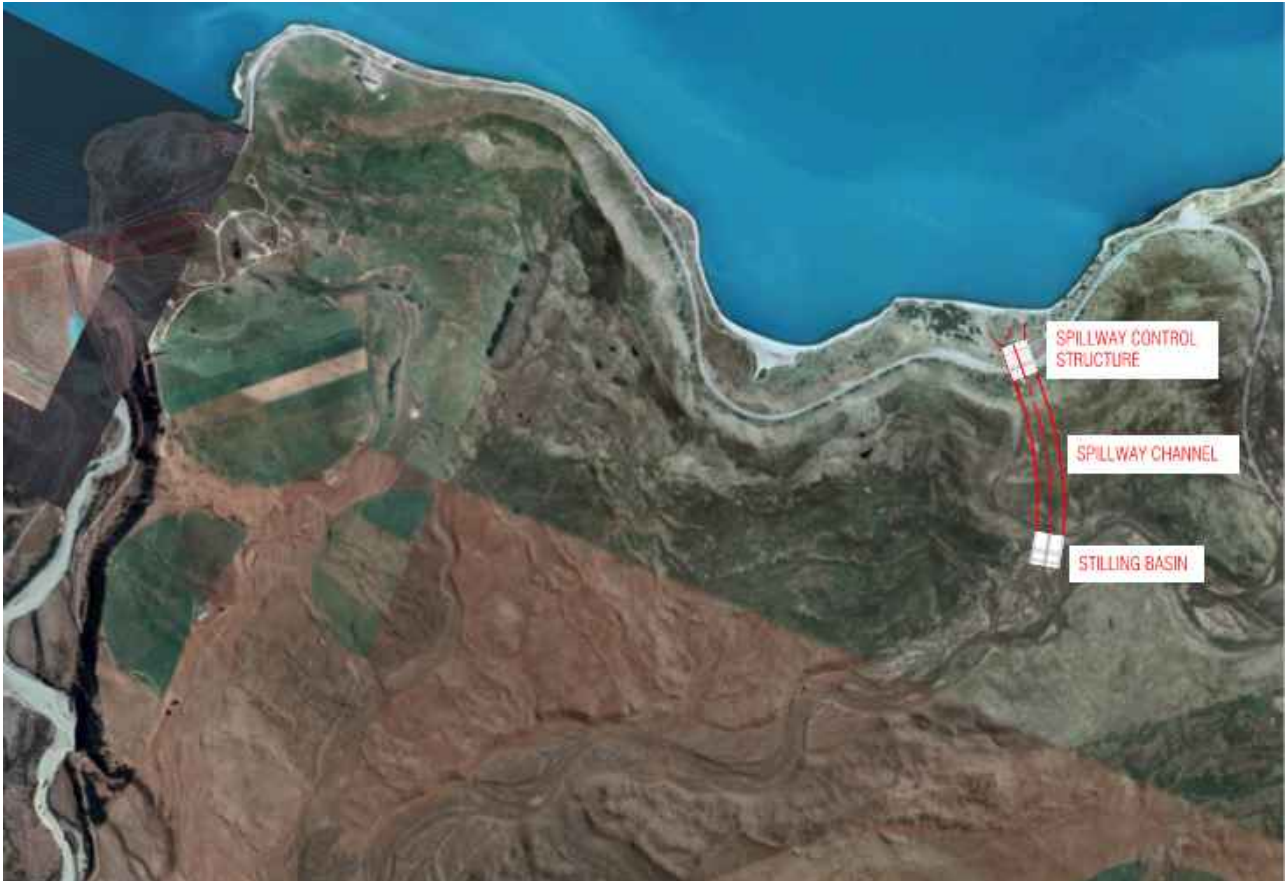
Figure 38 - Concept Spillway Arrangement
