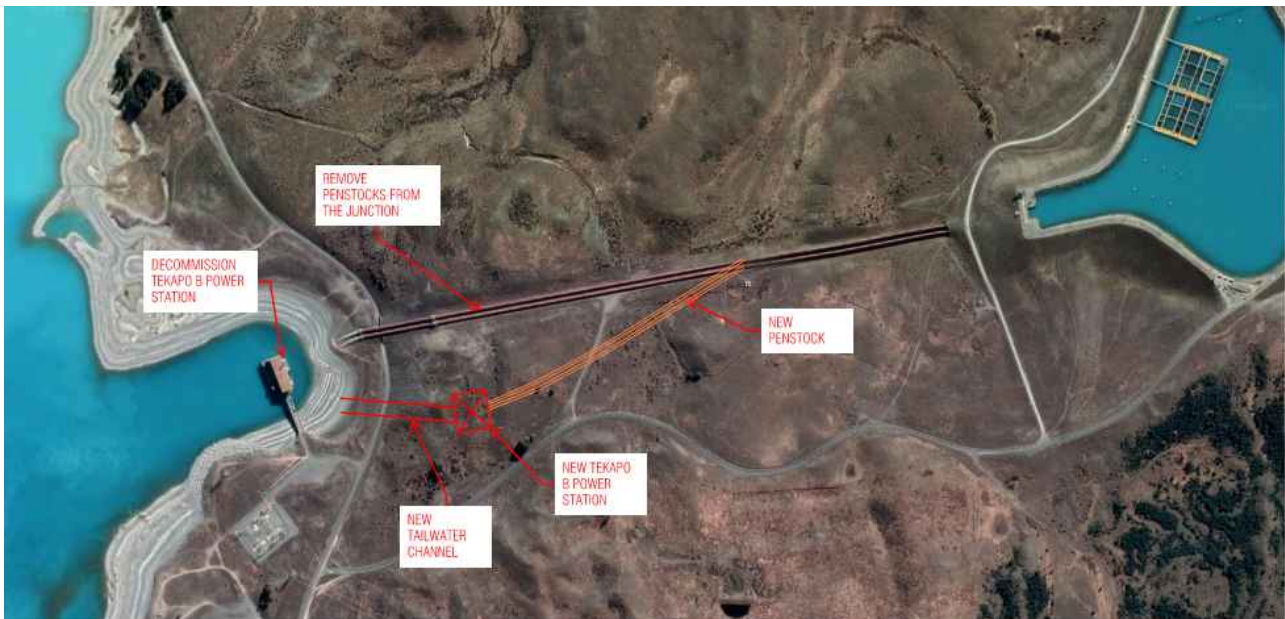
Figure 42 - Concept Replacement Tekapo B Power Station Layout
