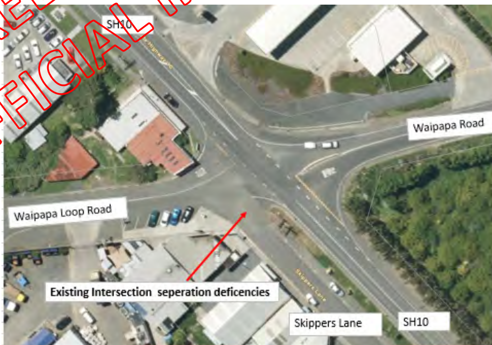
Figure 14: Existing intersection separation deficiencies
