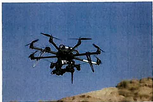
An unmanned aerial vehicle piloted by researchers uses a digital camera to take detailed photos of an outcrop's rocky layers in Spain. The flight was part of a reservoir modeling database project aimed at learning more about the fluid dynamics of similar subsurface rock formations. Photo courtesy of Simon Buckley/Aleksandra Sima.
