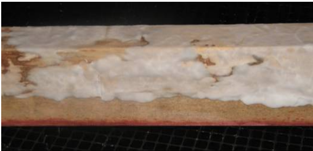
Figure 12 – HMC sample B31H/1, treated with boron on one edge, after 56 weeks exposure. Extensive mycelium on the untreated sides of the sample but associated decay was relatively shallow.
