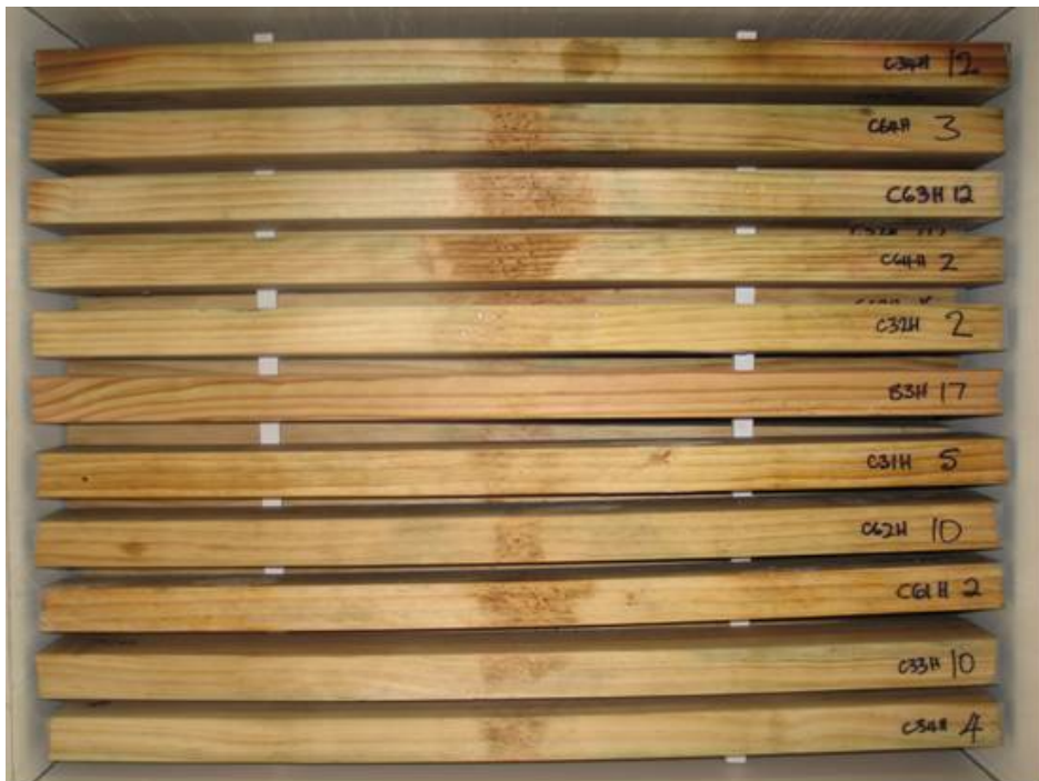
Figure 6 – Copper naphthenate treated HMC samples in tank 2, layer 3 (3 rd from bottom), after 56 weeks exposure. Samples were drier than in the top layer but there were still patches of fresh mycelium on the faces of samples that had been treated only on one or two edges.
