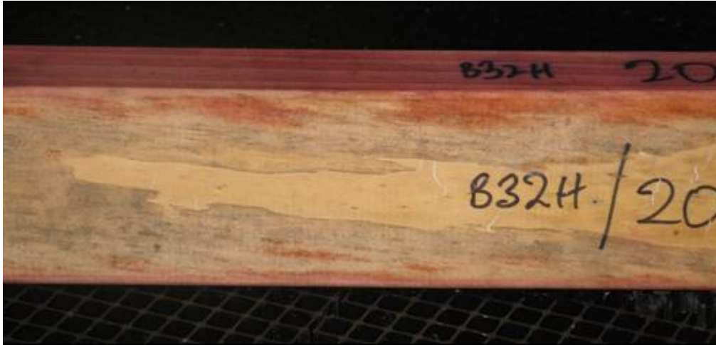
Figure 15 – HMC sample B32H/20, boron treated on two edges, after 56 weeks exposure. Decay and fine mycelium spreading on the faces between the treated edges at one end of the sample. This appears to have been from outside contamination and not the original Oligoporus placenta feeder block infection.
