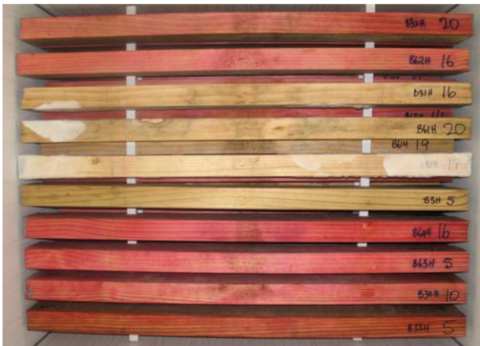
Figure 8 – HMC boron treated samples in tank 6, layer 4 (3 rd from top), after 56 weeks exposure. There was extensive fresh mycelium on the untreated surfaces of three samples that had been treated on only one edge. While there was extensive mycelium growth, decay in the samples was only light-moderate.
