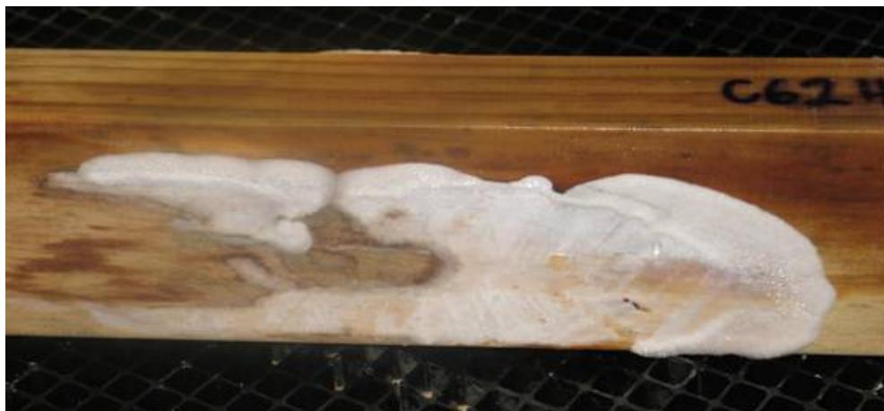
Figure 10 – HMC sample C62H/7, copper naphthenate treated on two edges, after 56 weeks exposure. There was extensive mycelium developing on the untreated faces around the original infected area but the wood underneath was still relatively sound. This sample was from the top layer in Tank 2. Nineteen of the 20 samples in this treatment group had fresh mycelium on the untreated surfaces.
