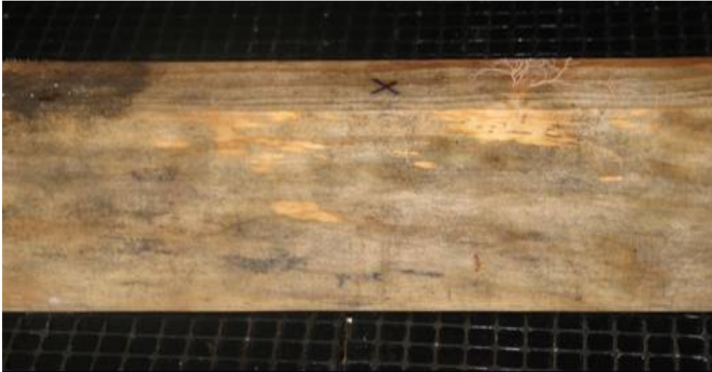
Figure 13 – Untreated sample (not pre-decayed) UMH/19, after 56 weeks exposure. Decay mycelium and pale discolouration associated with decay appeared to have come from outside contamination.
