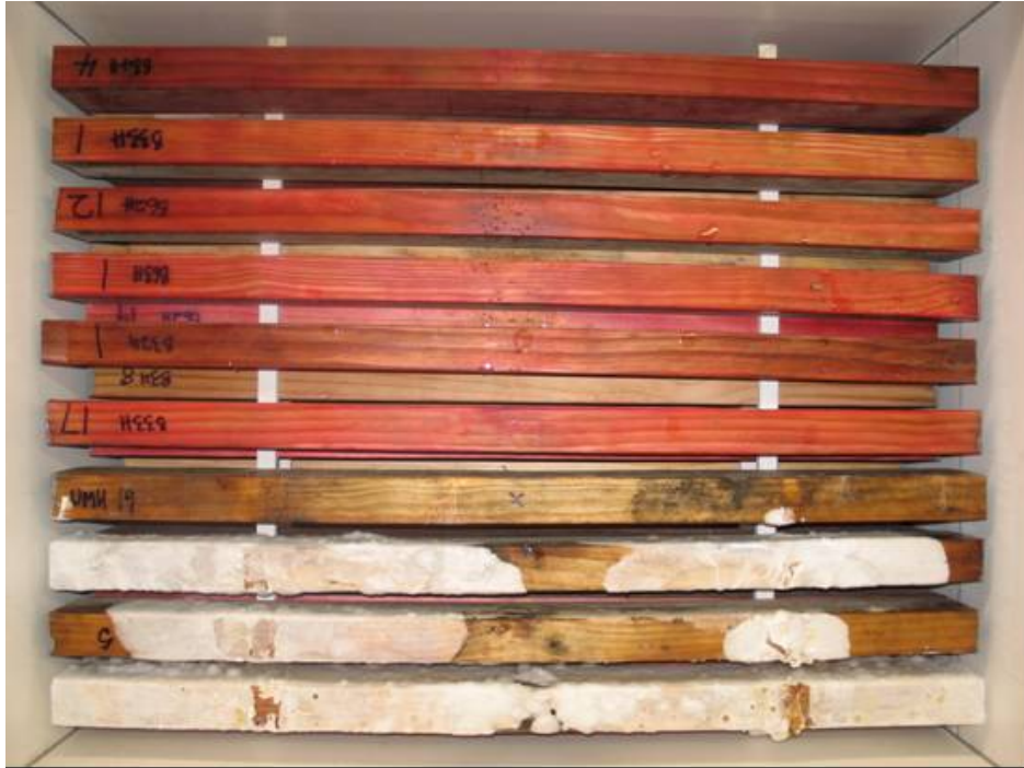
Figure 7 – HMC boron treated samples in tank 5, layer 6 (top), after 56 weeks exposure. There was extensive mycelium on the untreated surfaces of one control sample and two adjacent samples that had only been treated on the lower edge. Other treated samples in that layer were free from fresh decay.
