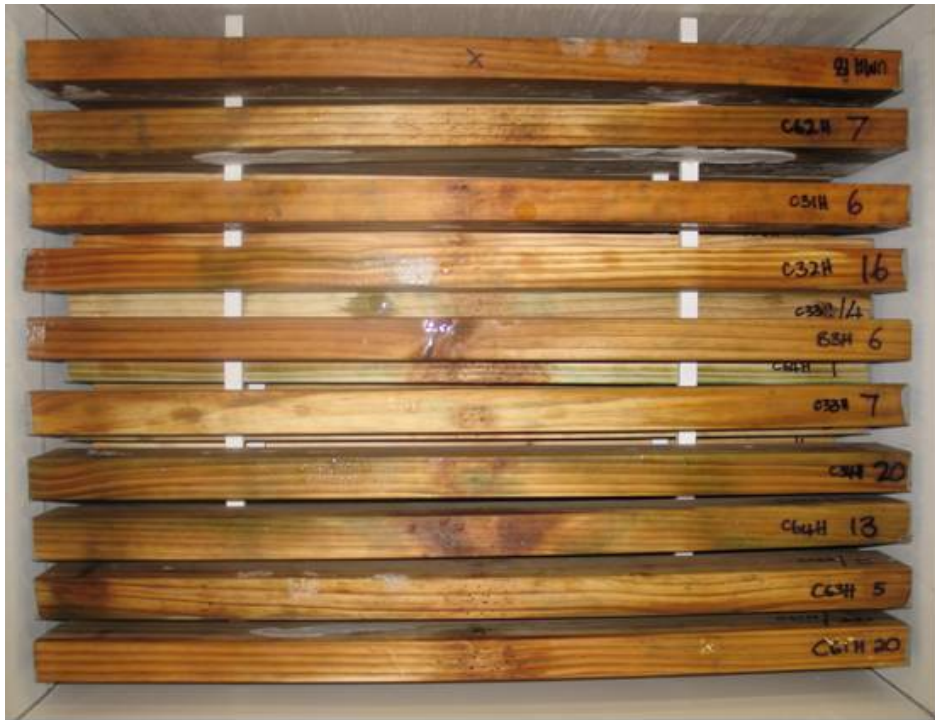
Figure 5 – Copper naphthenate treated HMC samples in tank 2, layer 6 (top), after 56 weeks exposure. There were patches of decay mycelium on the sides of most of the samples treated on one or two edges. Decay areas that had developed on the upper edge before treatment were still visible.
