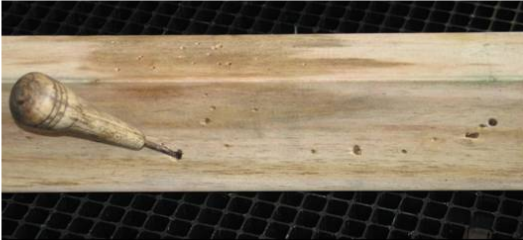
Figure 17 – LMC sample C62L7, copper naphthenate treated on two edges after 56 weeks exposure. Decay well established in patches on the untreated surfaces adjacent to and spreading out from the original feeder block infected area. There was no obvious mycelium and only minor colour changes on the surface to indicate that the wood was deteriorating. Deflection has increased in this sample by more than 20% since the 8-week assessment.
