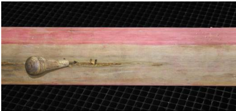
Figure 18 – LMC sample B62L/6, after 56 weeks exposure. Decay fruiting bodies and moderate decay between the treated edges but deflection had only increased by 12% since the first 8-week assessment. This sample was in the relatively damp bottom layer of the LMC stack.
