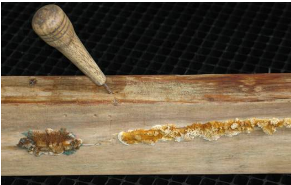
Figure 16 – LMC control sample U3L7, after 56 weeks exposure. Extensive fruiting bodies and decay in this sample due to damp conditions in the bottom layer of the stack. This sample failed during the deflection test of the 56-week assessment.
