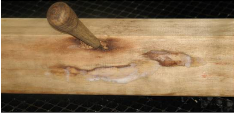
Figure 9 – HMC sample C32H/17, copper naphthenate treated on two edges, after 56 weeks exposure. Decay mycelium spreading from the original infected area and a deep internal decay pocket near the original decay feeder block site.
