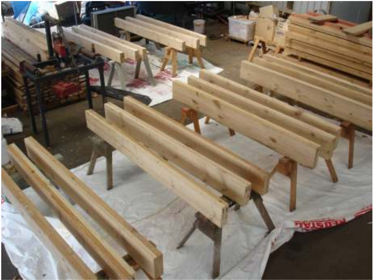
Figure 4: Assembled lintels prior to injection.
