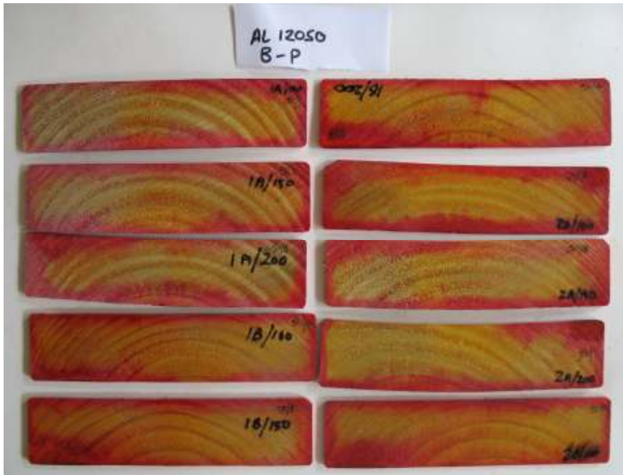
Figure 6: Penetration of boron for the 200x50 mm lintels. Sample A contained the injection holes.
