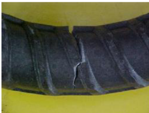
Figure 9: Fracture during straightening
