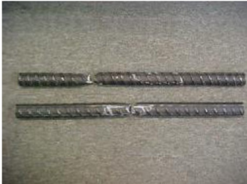
Figure 13: Examples of fracture location and cracks region as marked in white relative to bent section in the middle.
