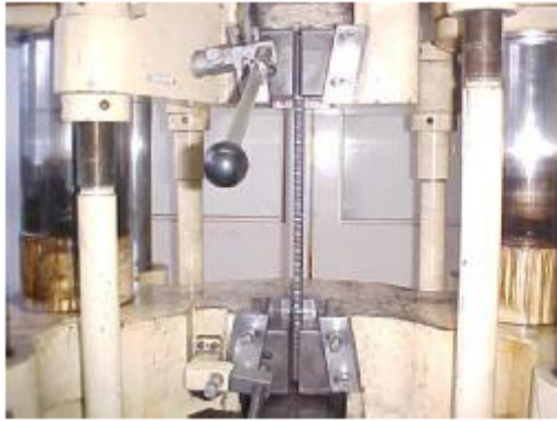
Figure 2: Tensile test set up
