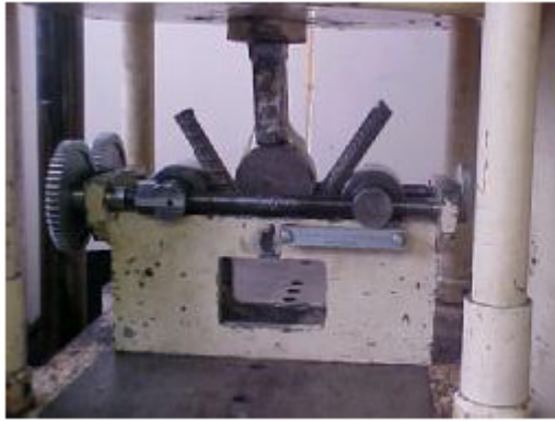
Figure 3: Guided bend jig set up
