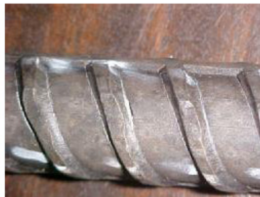
Figure 10: Example of surface cracks
