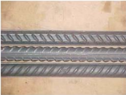
Figure 6: Amsteel bars consist of two rows of crescent shaped transverse ribs reversing in direction on opposite sides of the bar with two additional longitudinal ribs on one side. On the other side there is one longitudinal mark joining two consecutive ribs, spaced at 1m apart.
