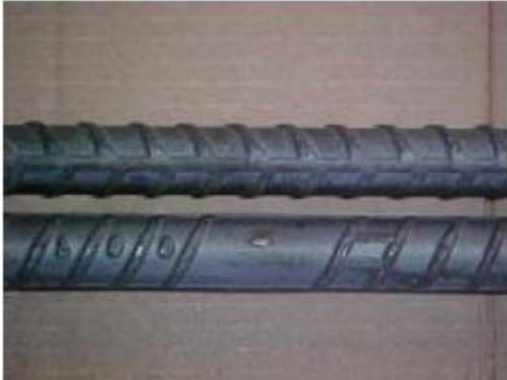
Figure 8: Pacific Steel bars can be identified by two rows of uniform height transverse ribs reversing in direction on opposite sides of the bar and have on one sides, two missed deformations adjacent to two additional longitudinal bars joining two consecutive ribs. There is alphanumeric marking "SEISMIC 500" adjacent to the missed deformations spaced at 1m apart.
