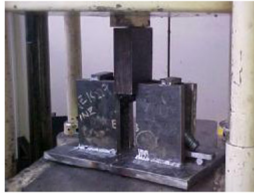
Figure 4: Reverse guided bend jig
