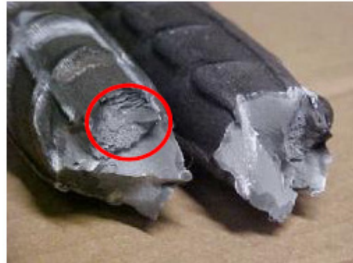
Figure 14: Cracks leading to fracture as marked
