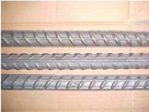
Figure 7: Natsteel bars consists of two rows of transverse ribs reversing in direction on opposite sides of the bar with 3 additional longitudinal ribs - one on one side and two on the other. On the sides with two longitudinal ribs, there are two longitudinal marks deformed in between two consecutive ribs, spaced at 1m apart.
