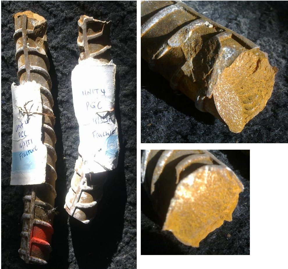
Figure 6 - Item 4 - Orange marked #10 bars samples shown in Figure 5 with flat running fractures initiating from surface abrasion marks likely caused during deconstruction.
