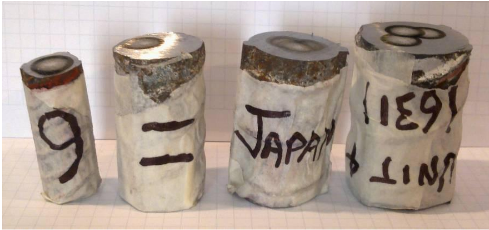
Figure 14 - PGC bar samples after chemical analysis
