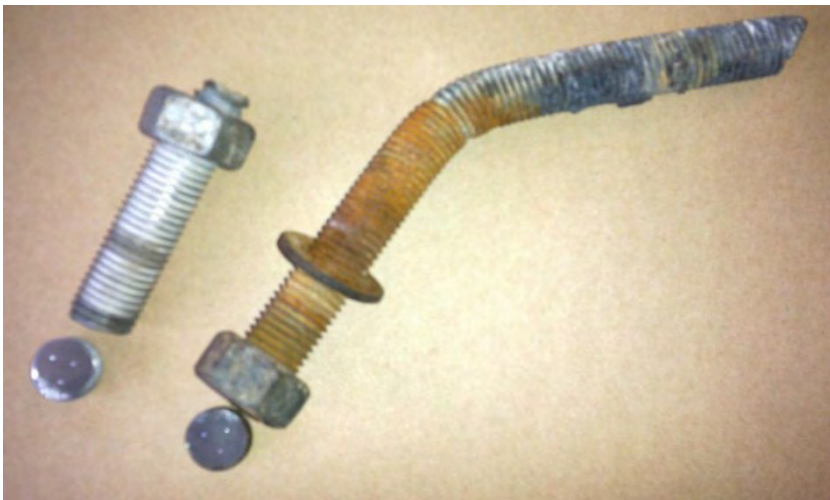
Figure 38- M20 Property Class 5.8 threaded studs from Drag Bars after hardness testing by MTL (Figure 62)
