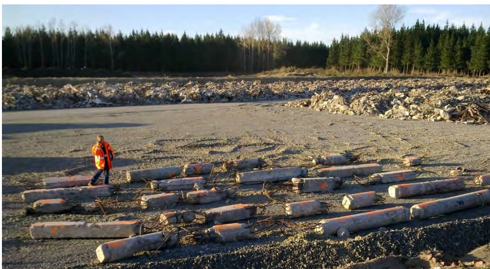
Figure 48 - CTV Columns remnants extracted from the Burwood Landfill CTV debris (at right) for Schmidt Hammer testing and coring. Full height and partial height remnants can be seen.
