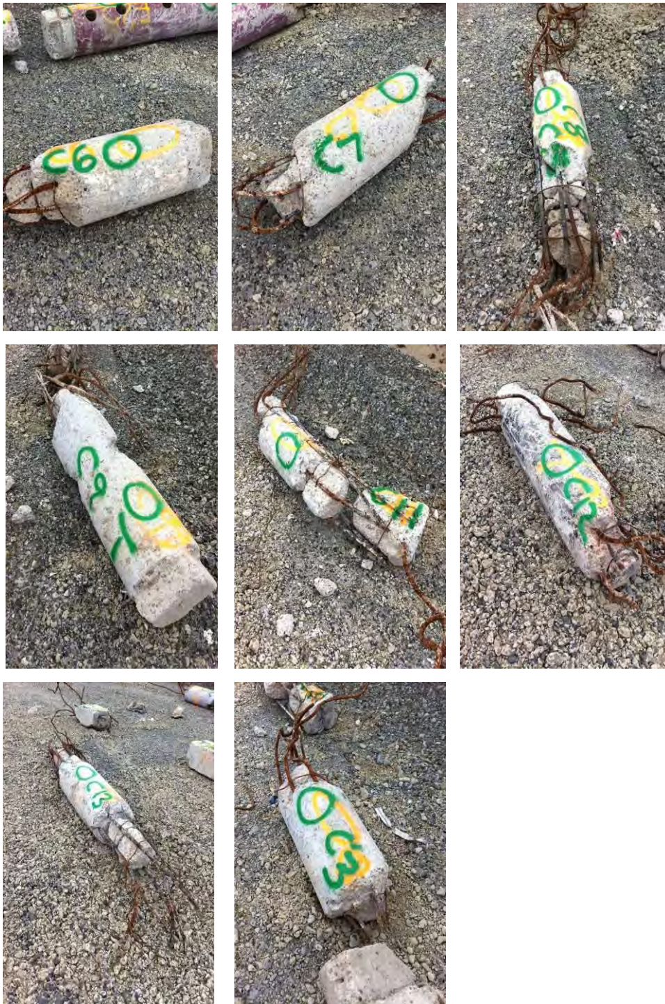
Figure 53 -400 mm Diameter Columns at Burwood showing similar base and/or mid-height failures (Left to right, top row down) (a) Test item tC6 Level 6 column head with mid-height failure; (b) tC7 with base and mid-height failures; (c) tC8 with base flexural (near end) and mid-height spearhead failures; (d) tC9 Level 6 column head with mid-height failure; (e) tC11 base (near end) and mid-height failure; (f) tC12 base and mid-height failure; (g) tC13 base and mid-height flexural failure (near end); (h) tC3 similar to tC13 but lower bars have been cut during de-construction at start of spalling.
