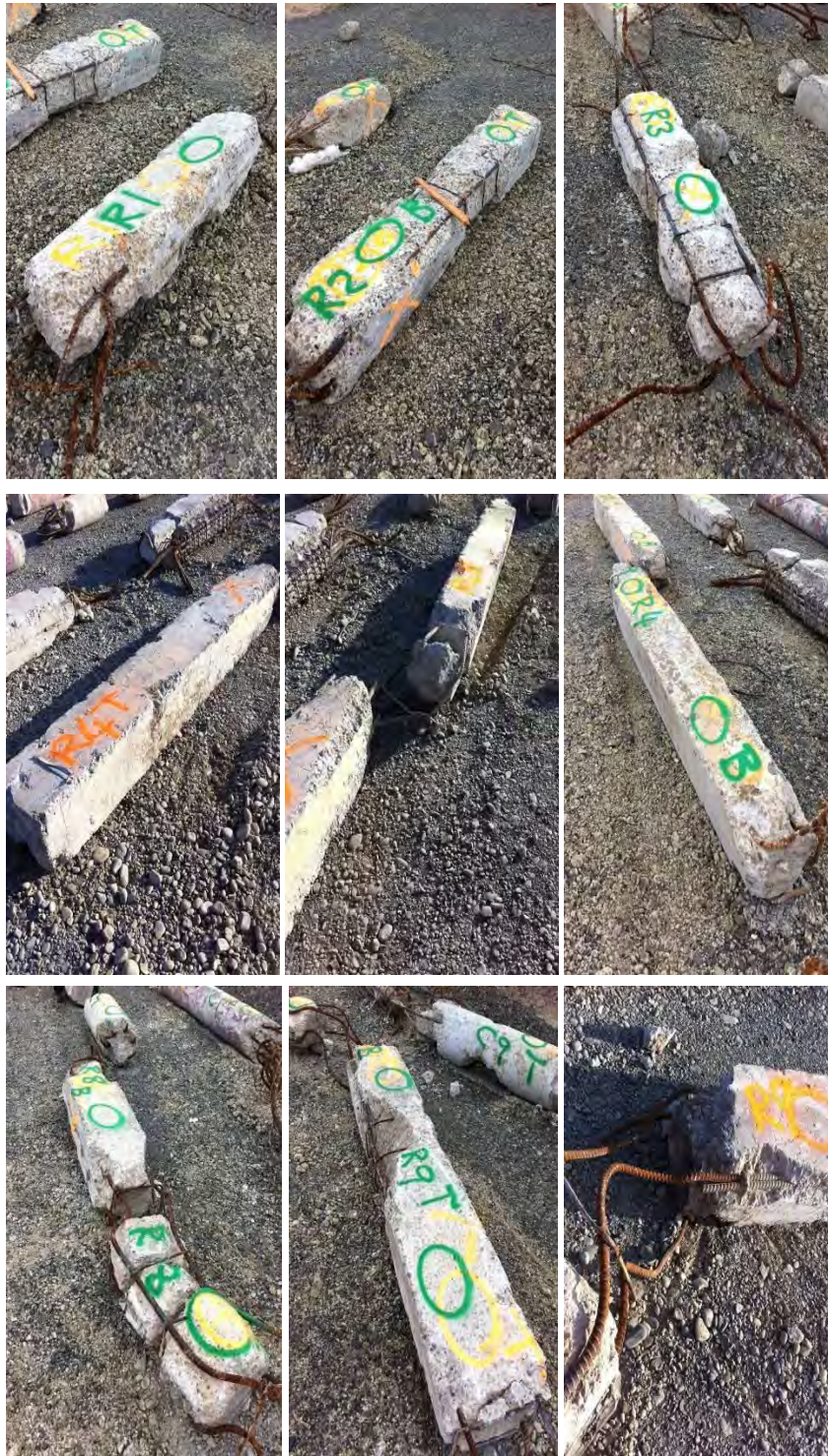
Figure 55 -400 x 300 mm Rectangular Columns (Left to right, top down) (a) tR1 beam-column joint failure at base, mid-height failure; (b) Level 6 to Roof base or beam-column joint failure; (c) tR3 failure base and top; (d) tR4 Level 6 to Roof with beam-column joint failure, still connected by rebar to (e) tR4' below which also (f) indicates beam-column joint failure at tR4' base (near camera); (g) tR8 with damage from mid-height still connected to tR9 above (h) with beam-column joint failure with (i) underside of tR9 smooth.
