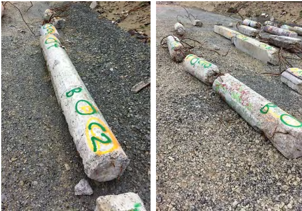
Figure 54 - Level I Entry 400 mm Diameter Columns (left to right) (a) Test item tC2, 6-D12 vertical bars fractured at base (DENG Dwg S14 C23); (b) Item tC10 with down pipe cast in (DENG Dwg S14 C21 or C22)
